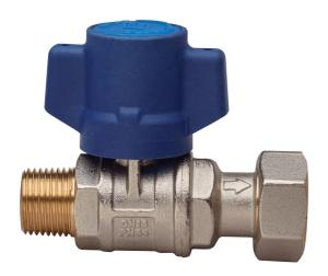
Full bore ball valve for water meter entry, male threaded/nut connection, check valve incorporated, with anti-tampering T-handle and ball with automatic rinsing system.
