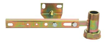
Steel cross beam, center distance 250 mm, with threaded union tail EN 10226-1 and triangular fixing plate for raw plugs.
